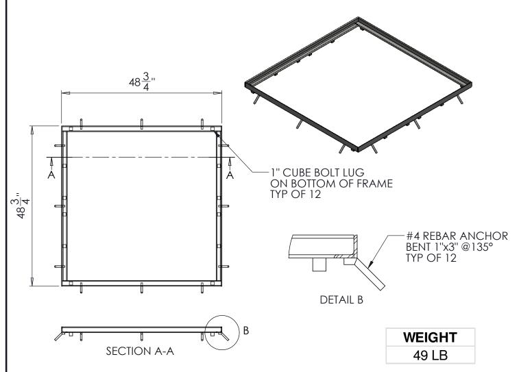
IF TREE GRATE IS TO BE BOLTED TO TREE GRATE FRAME: ORDER SBF ID#D00BD "BOLT DOWN KIT". EACH KIT CONTAINS:
